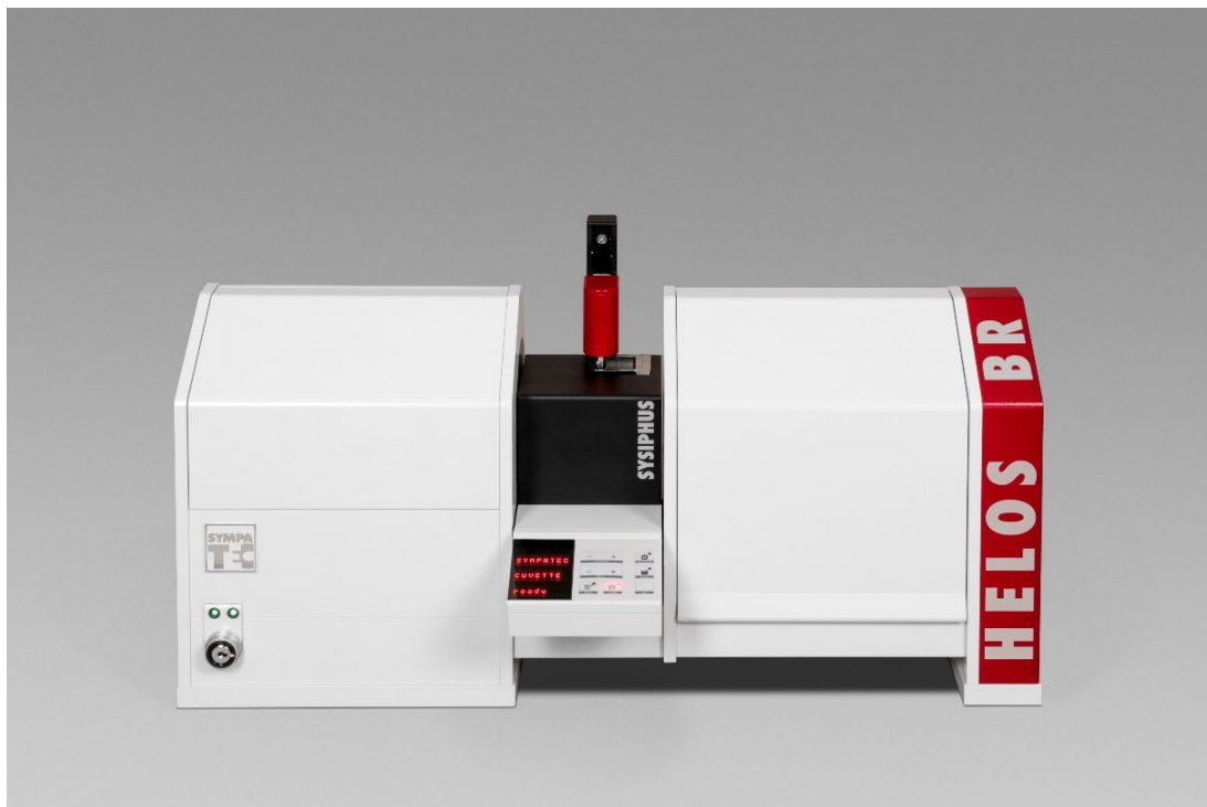
Figure 1: HELOS/BR laser diffraction sensor with CUVETTE/SYSIPHUS wet disperser for particle size analysis of suspensions and emulsions.
